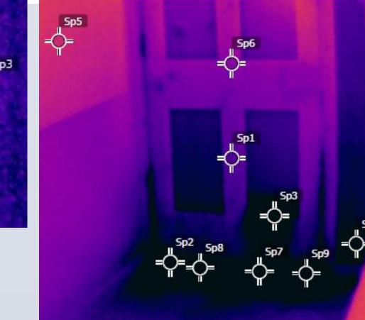
Fig 10 (above). Cold drafts are easy to spot (here, issuing inside under a museum door) and this can help to identify where pests
