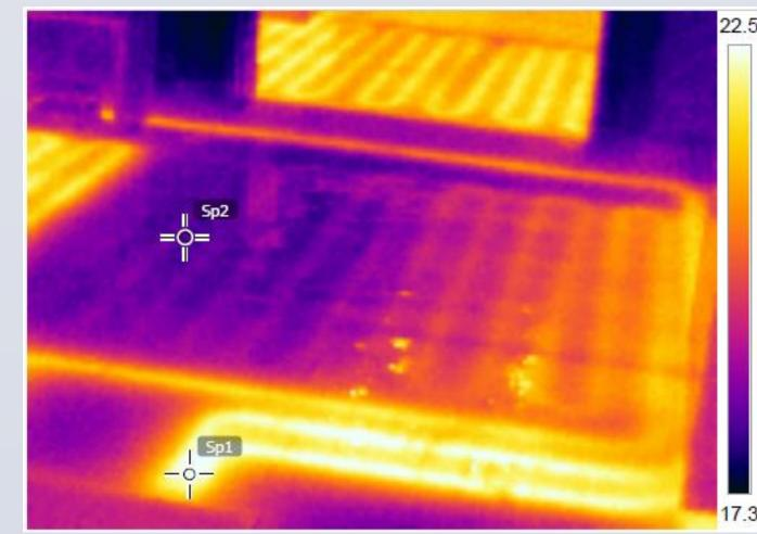
Fig 8 (above). Not only is underfloor heating very easily assessed to check if it is working (here, above, a section has failed), but the locations of the hot water pipes can be recorded in some detail so that specimens or display cases can be sited more appropriately in the future, to reduce the chances of damage by overheating.
