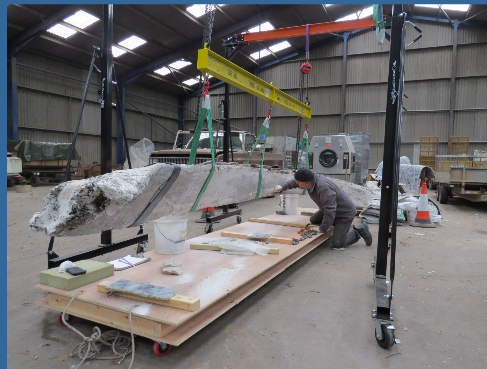
Figure 3, below. The bones were lifted and turned using gantries, chain hoists and cloth slings.
