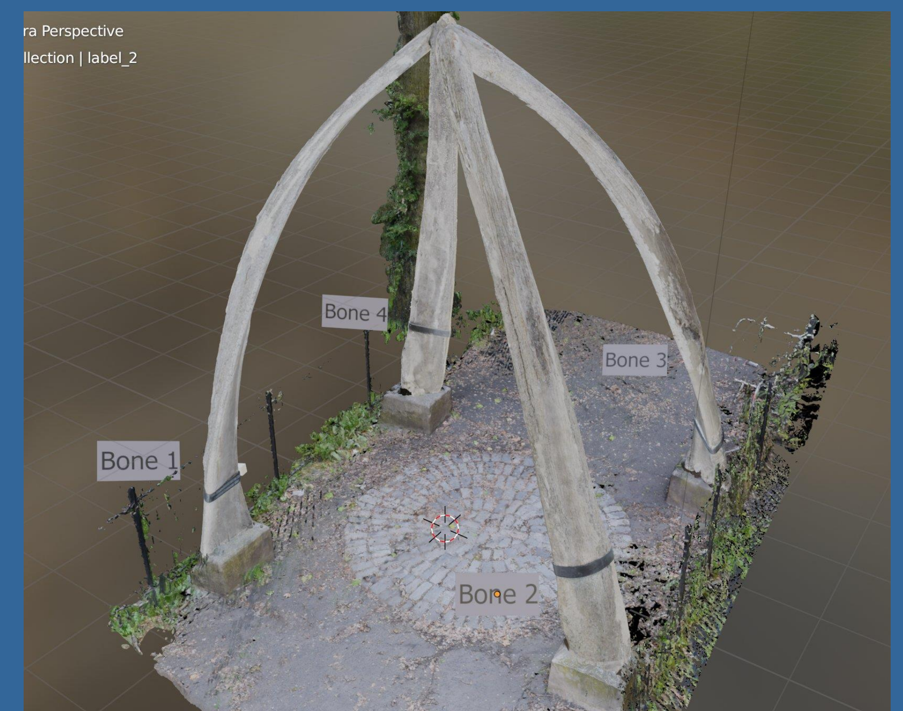
Fig 9, above. The whale bones after conservation work and 3D scanning, digitally reconstructed as a 3D digital model of the arch.
